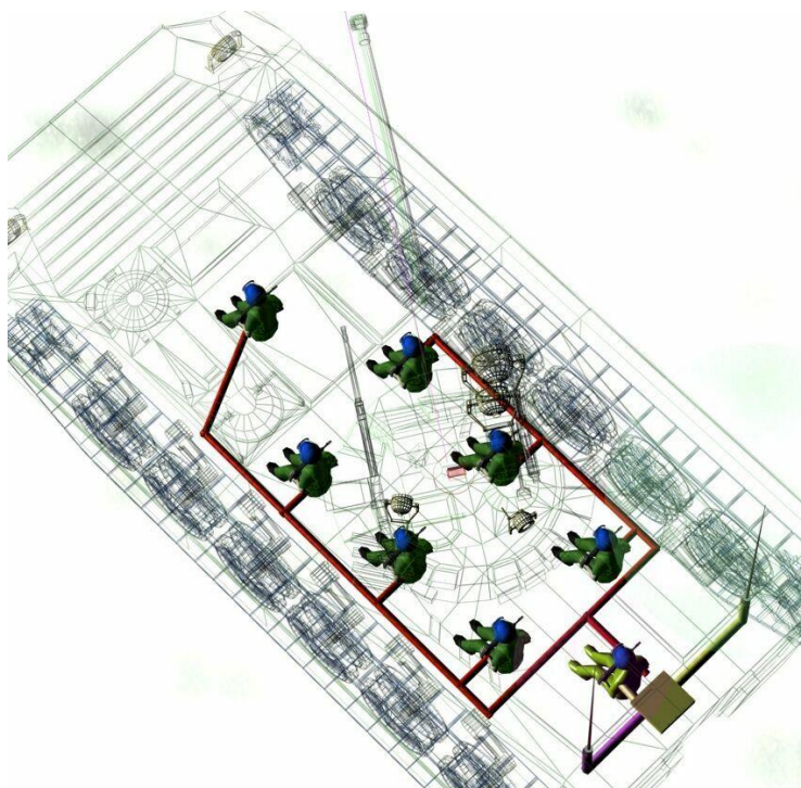
Fig. 3 Internal connection of Body LAN in armored military vehicle
